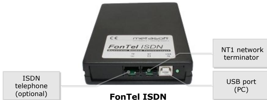
**FonTel ISDN** recorder is connected to the network terminator NT1 (S0 interface) similarly to an ISDN telephone. NT1 network terminator has at least 2 outputs for connecting, for example, two ISDN telephones. If any of the sockets is available, the recorder's **NT** input can be connected to it. If all of the sockets are in use, one of the connected devices shall be plugged out, the recorder (**NT**) is placed instead, and the plugged-out device is connected to the recorder's **TE** socket.
