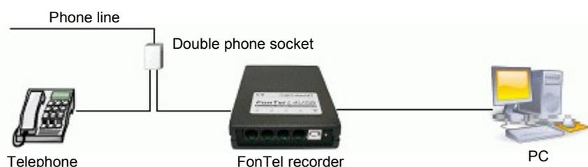
Example of connecting the recorder to a phone line that ends with a double phone socket
