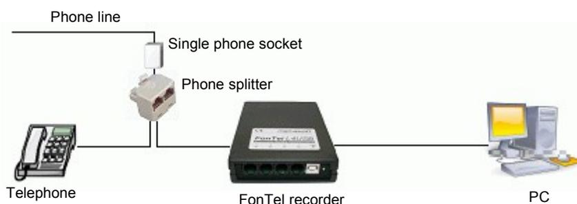
example of the recorder's connection through a phone splitter to a phone line that terminates with a single phone socket
